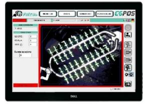
**<u>E6 FALCON</u>** responds to the need to verify the completeness of the piece at the moment it is produced. Typical applications are metal or plastic material **moulding**, **die casting** and **thermoforming**.
